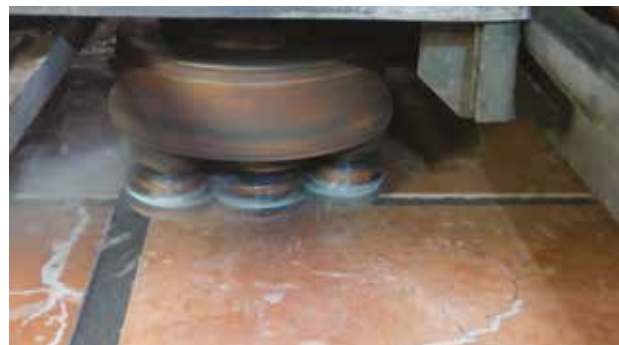
The satellite system for lapping tiles in parallel rows
