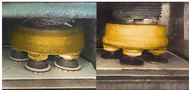
By choosing PREMIER satellite heads on a lapping line, replacing only the tool, it is transformed from a simple lapping machine into a calibrating / polishing / lapping machine.
