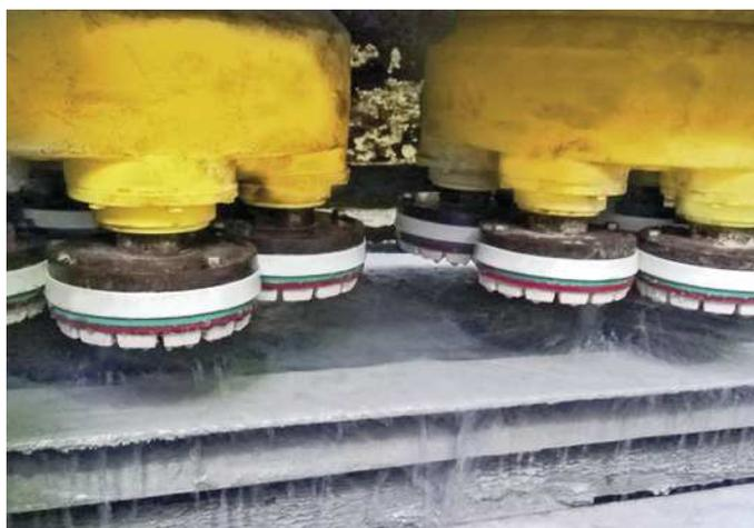
The Satellite System is also an **optimal solution for dark colours**, as tools with a finer grain can be used while maintaining the same removal rate, resulting in scratch-free tiles with a higher gloss level.
